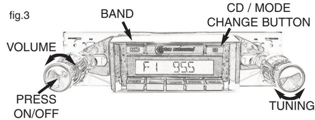
3. Depress the CD button (4) to toggle the functions of the radio .The sequence displayed will be : Radio—USB—CDC—AUX—Radio.
